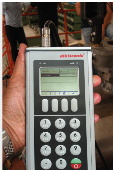
alkitronic ® cardos OP Operation interface with LC Display and menu guidance • Remote control to start/stop the cycle • Choose of parameter settings • Data transmitting via USB
